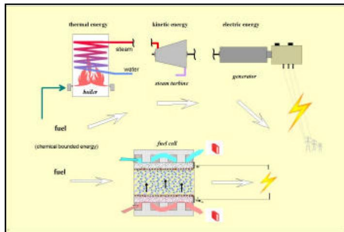
figure 1: principles of the electricity generation with water/steam cycle and with the fuel cell
