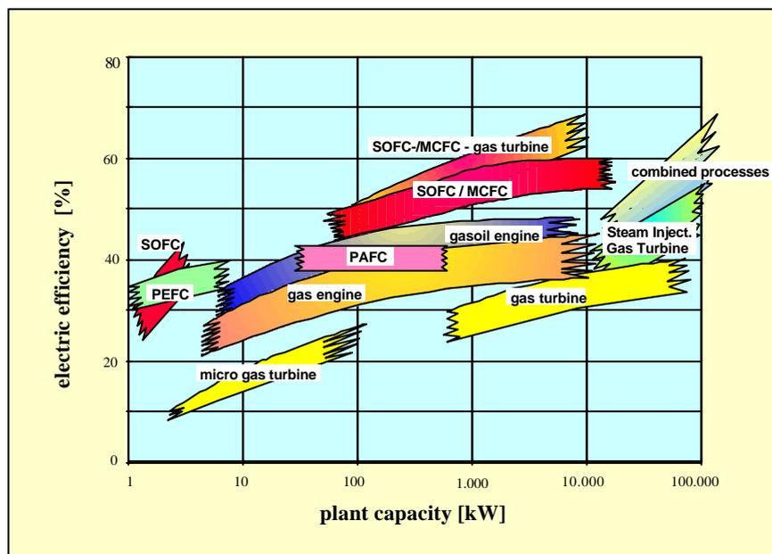
figure 5: relation between plant capacity and electric efficiency
