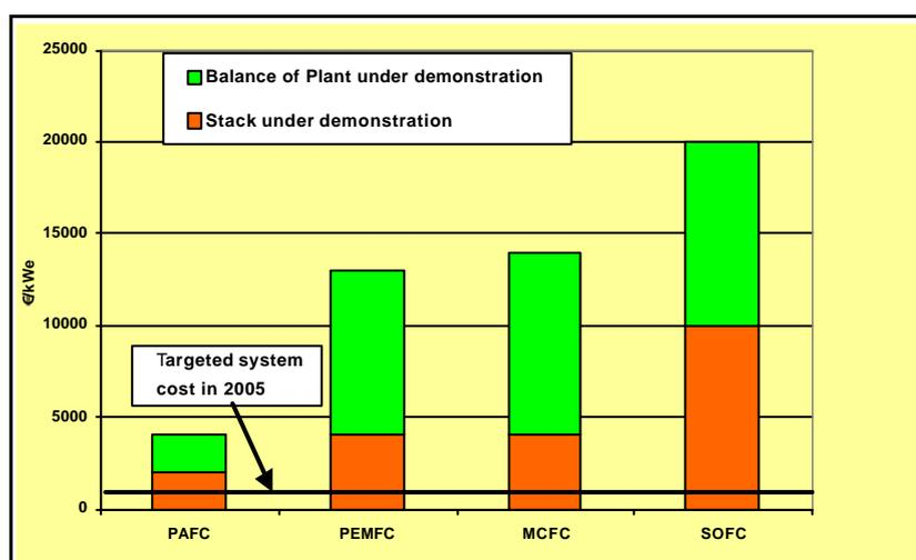
figure 9: specific cost under construction for industrial demonstration units
