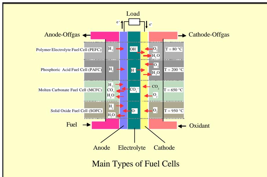
figure 2: main fuel cell types and their characteristics
