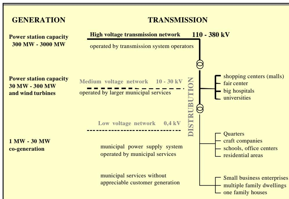
figure 11: structure of the European electricity network, generation, transmission and distribution
