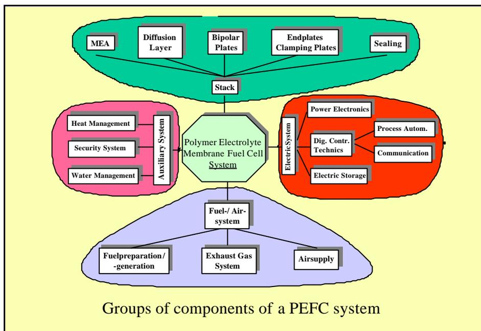
figure 4: main components of a PEFC-system
